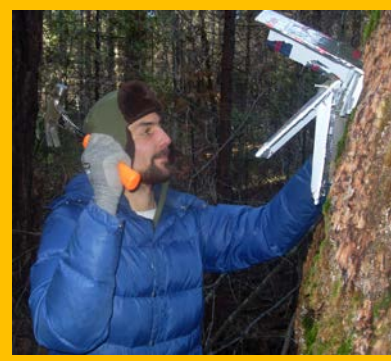
Figure 3. Tom Reyes, Yosemite National Park (Yosemite) volunteer, deploys a climate sensor with a solar radiation shield to collect micro-scale climate data.
