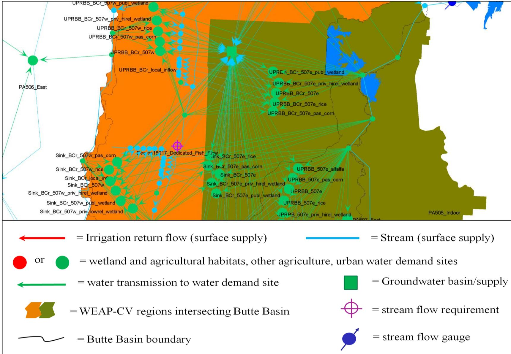
Figure 2. water supplies, demands, and delivery in a portion of Butte Basin represented in WEAP as a system of links and nodes.
