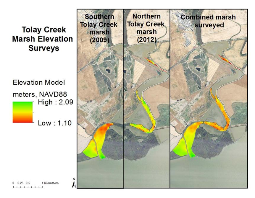
Figure 6. DEMs for 2009 (mouth) and 2012 (upstream) elevation surveys at Tolay Creek.
