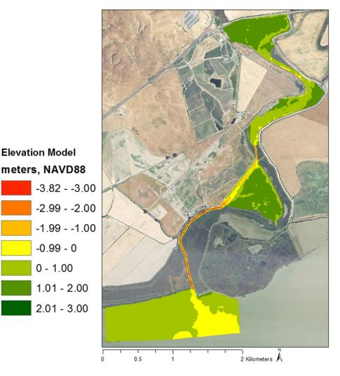
Figure 16. Bathymetric survey of Tolay Creek and adjacent shoals.
