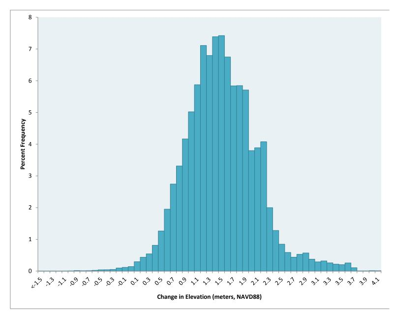
Figure 25. Change in elevation of Tolay Creek mudflat between 2000 and 2012.
