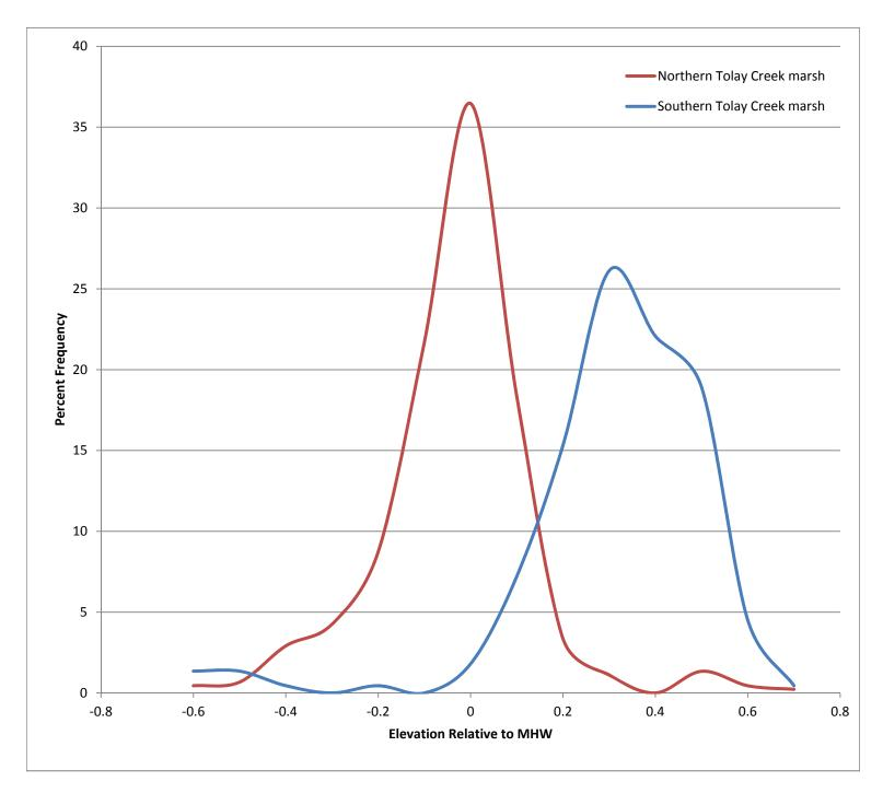
**Figure 14**. Percent frequency of Tolay Creek elevation points taken at the southern mouth section that was inundated less frequently than the northern upstream section relative to MHW measured at nearby mouth (MHW=1.47) and upstream (MHW=1.62) water level loggers.
