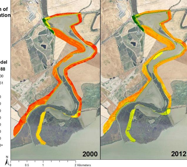
Figure 30. Digital elevation model of Tolay Creek upland comparing 2000 to 2012.
