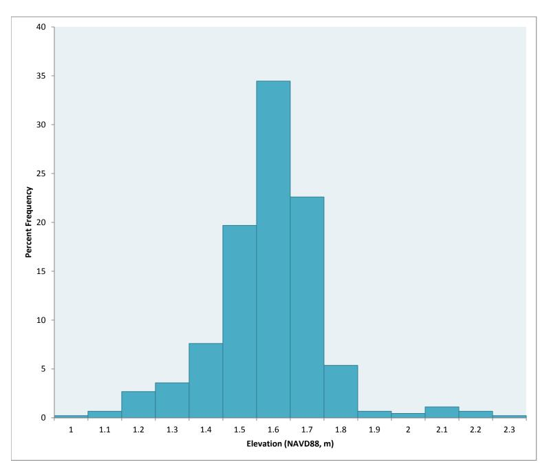
**Figure 11**. Percent frequency of marsh RTK GPS elevation points (meters, NAVD88) measured during 2012 at northern Tolay Creek upstream marsh.
