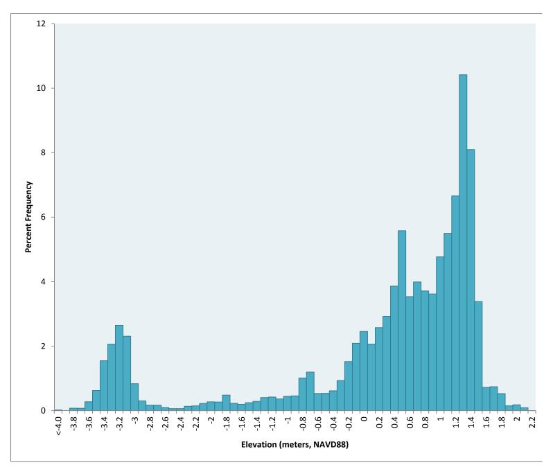
Figure 17. Percent frequency of bathymetric measurements of Tolay Creek and adjacent shoals during 2012 surveys (meters, NAVD88).
