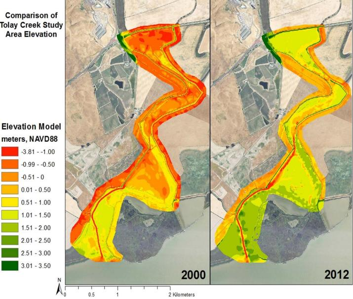
Figure 22. Digital elevation model of Tolay Creek study area comparing elevation between 2000 and 2012.
