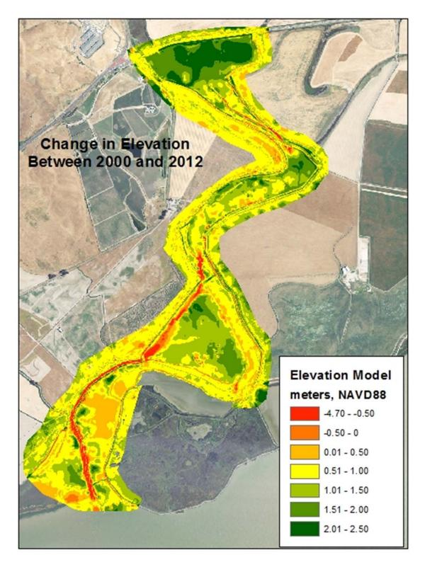
**Figure 23.** Digital Elevation model showing elevation change for the entire Tolay Creek study area between 2000 and 2012.
