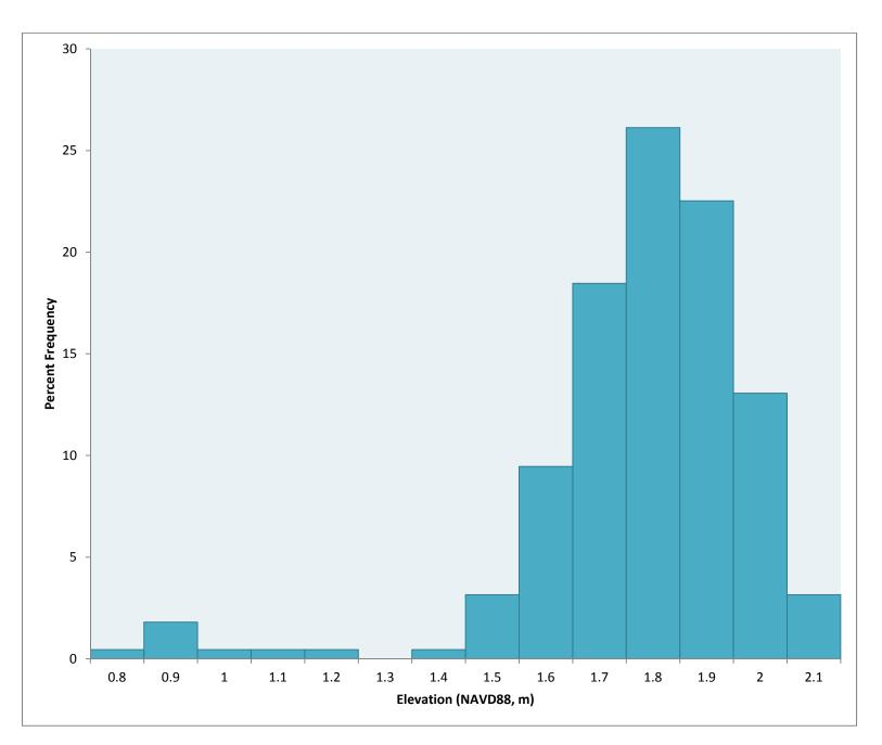
Figure 9. Percent frequency of marsh elevation points measured by RTK GPS (meters, NAVD88) at the Tolay Creek mouth.
