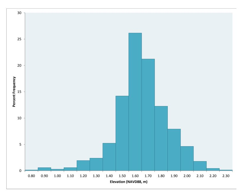
Figure 7. Percent frequency of RTK GPS elevation points (meters, NAVD88) for the Tolay Creek marsh plain.
