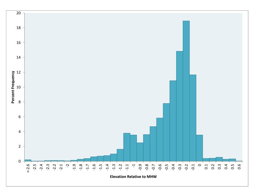
Figure 20. Percent Frequency of elevation measurements of Tolay Creek mud flats relative to MHW (MHW=1.54, average between upper and lower Tolay Creek water level loggers).
