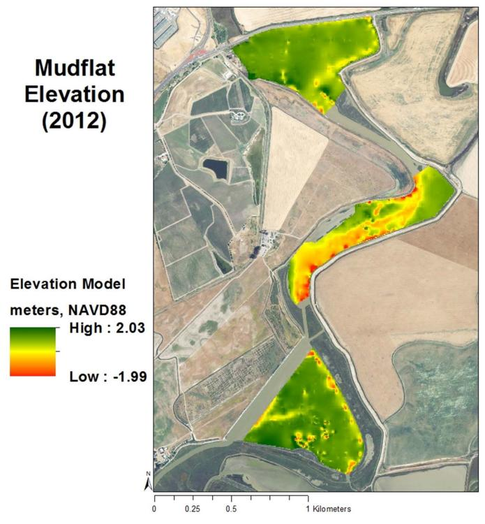
Figure 19. DEM of Tolay Creek mudflats created from 2012 bathymetric survey.
