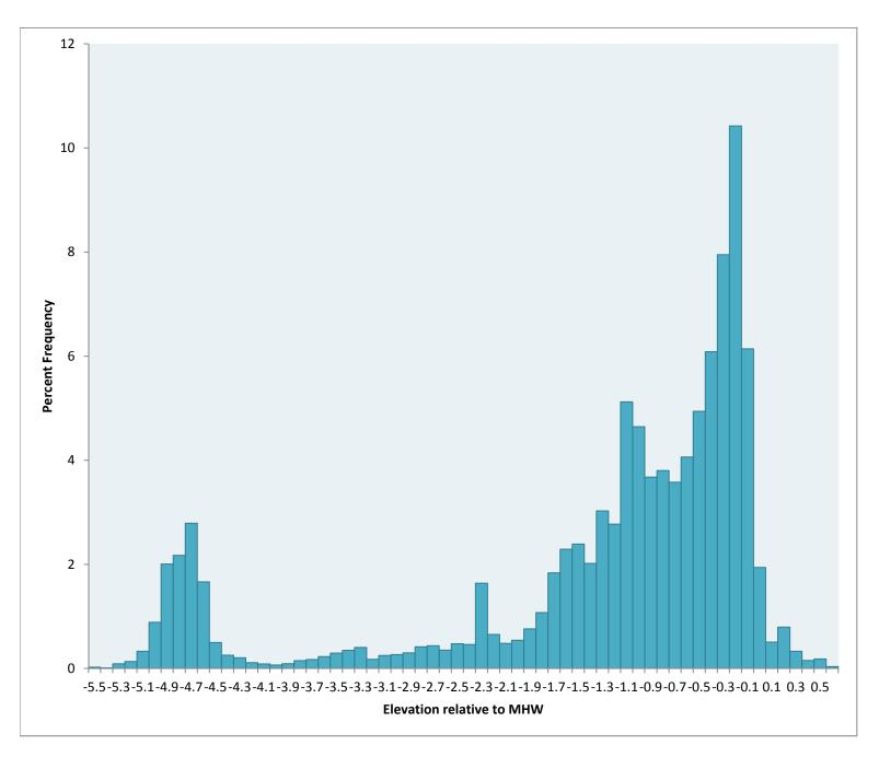
**Figure 18.** Percent frequency of bathymetric measurements of Tolay Creek and adjacent shoals during 2012 surveys relative to MHW (meters, NAVD88).
