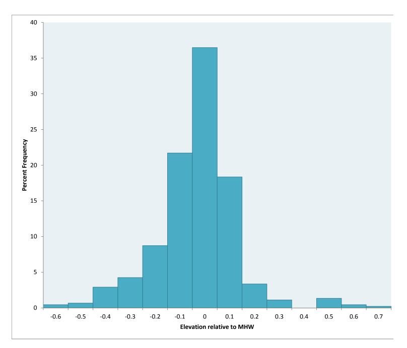
**Figure 12**. Percent frequency of marsh RTK GPS elevation measurements taken during 2012 at northern Tolay Creek marsh relative to MHW measured at northern Tolay Creek logger (MHW=1.62).
