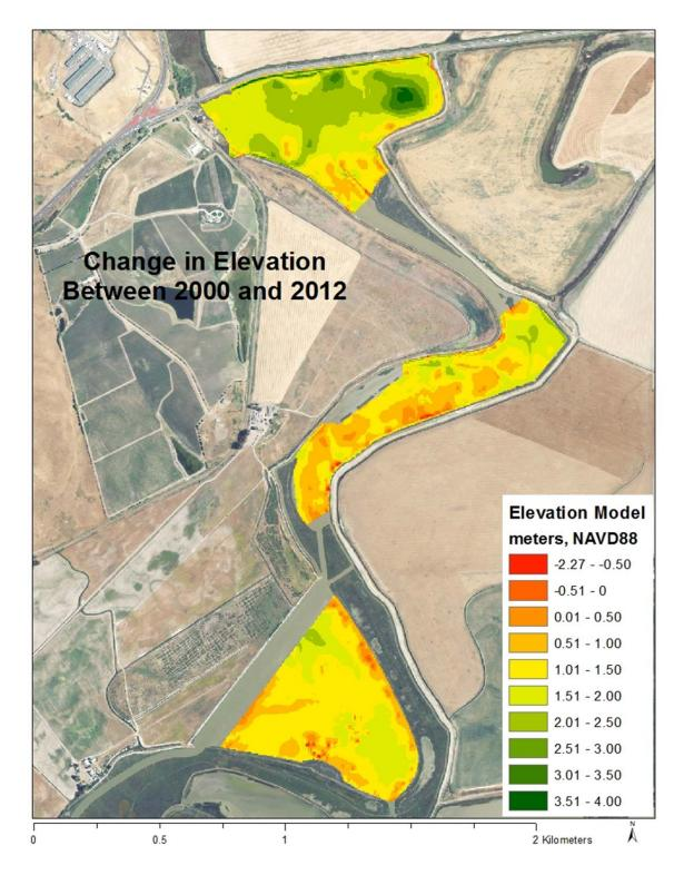
**Figure 26**. Digital elevation model of Tolay Creek mud flats showing elevation change between 2000 and 2012. Overall mud flats increased in elevation especially in the northern lagoon.
