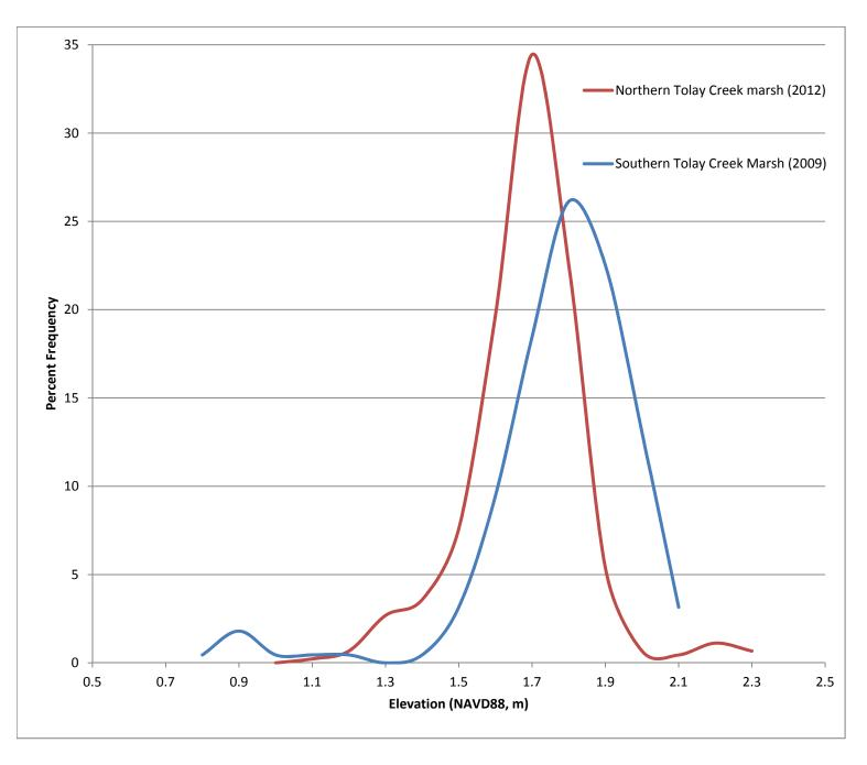
Figure 13. Comparison between southern mouth and northern upstream marsh elevation measurements (meters, NAVD88) at Tolay Creek.
