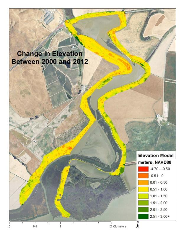
Figure 32. Digital elevation model of Tolay Creek upland showing elevation change from 2000 to 2012
