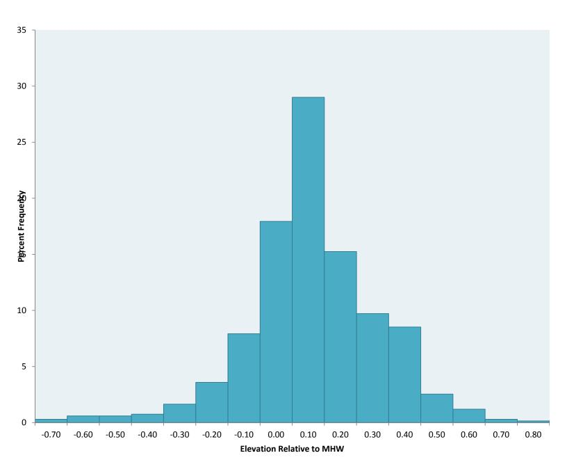
Figure 8. Percent Frequency of all marsh RTK GPS elevation measurements taken relative to an averaged MHW of the upper and lower Tolay Creek water level loggers (MHW=1.54 m).
