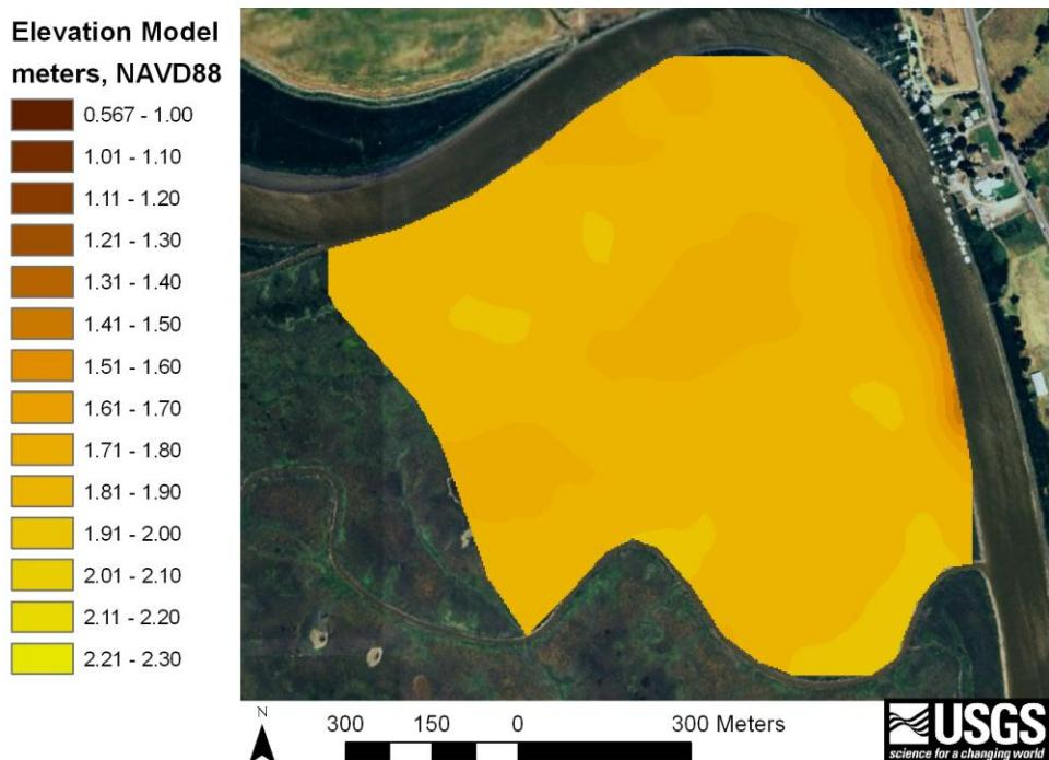
**Figure K-3.** Elevation model (3-m resolution) developed from ground RTK GPS elevation data.
