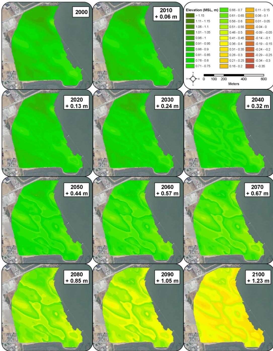
**Figure J-7.** WARMER results for Laumeister. WARMER accounts for changes in relative sea-level, subsidence, inorganic sediment accumulation, above/below ground organic matter productivity, compaction, and decay. Non-linear sea-level rise projections for California were used (Cayan *et al.* 2009).
