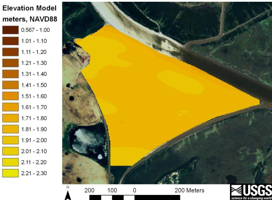
**Figure I-3.** Elevation model (3-m resolution) developed from ground RTK GPS elevation data.
