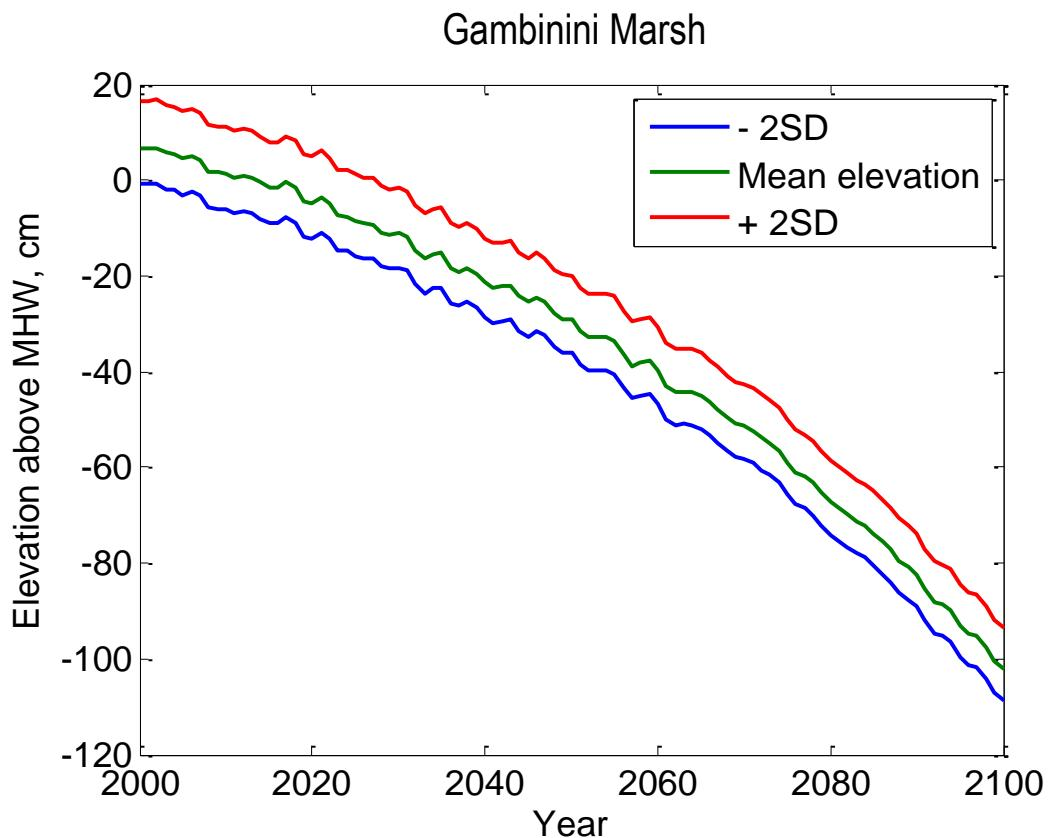
**Figure I-7.** Modeled scenarios of marsh elevation change for Gambini. Elevation above MHW is plotted versus model year.
