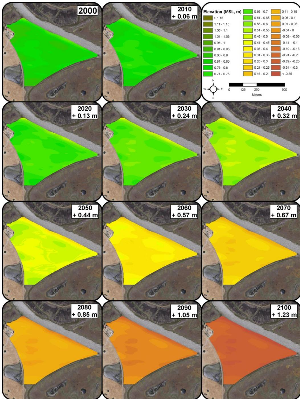
**Figure I-6.** WARMER results for Gambini. WARMER accounts for changes in relative sea-level, subsidence, inorganic sediment accumulation, above/below ground organic matter productivity, compaction, and decay. Non-linear sea-level rise projections for California were used (Cayan *et al.* 2009).
