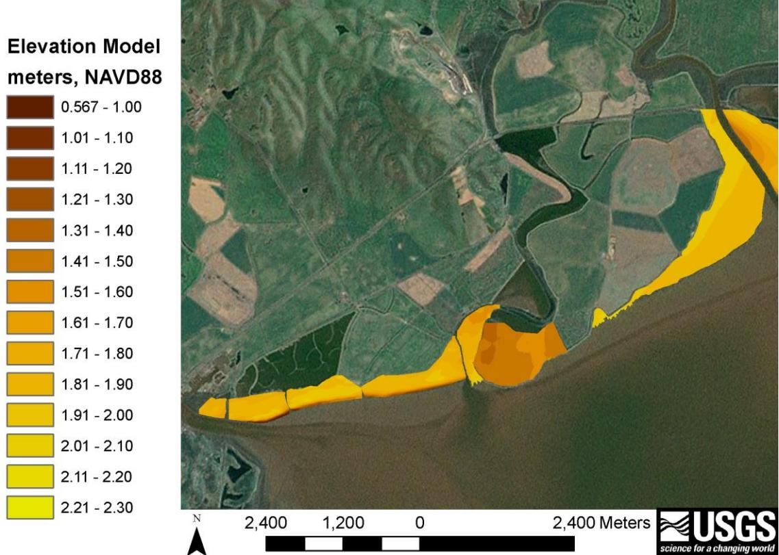
**Figure L-4.** Elevation model (3-m resolution) developed from ground RTK GPS elevation data for west San Pablo.
