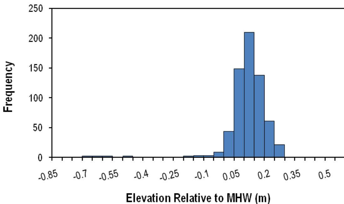
**Figure K-2.** Distribution of elevation samples relative to local mean high water (MHW) at Petaluma Marsh.
