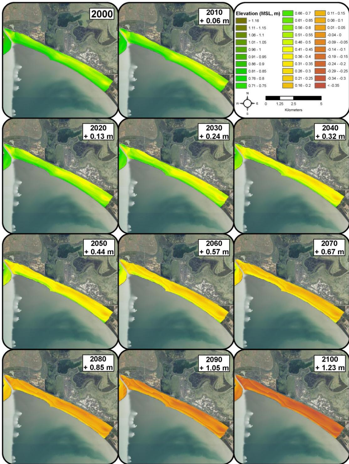
**Figure L-10.** WARMER results for east San Pablo. WARMER accounts for changes in relative sea-level, subsidence, inorganic sediment accumulation, above/below ground organic matter productivity, compaction, and decay. Non-linear sea-level rise projections for California were used (Cayan *et al.* 2009).
