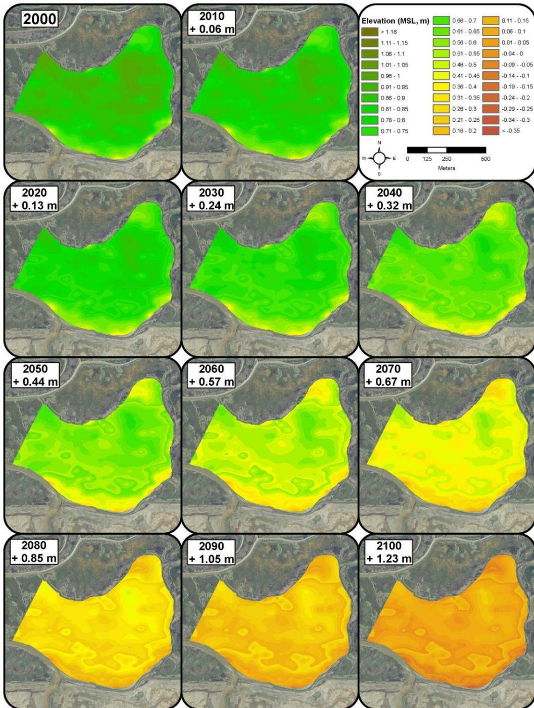
**Figure H-6.** WARMER results for Fagan. WARMER accounts for changes in relative sea-level, subsidence, inorganic sediment accumulation, above/below ground organic matter productivity, compaction, and decay. Non-linear sea-level rise projections for California were used (Cayan *et al.* 2009).
