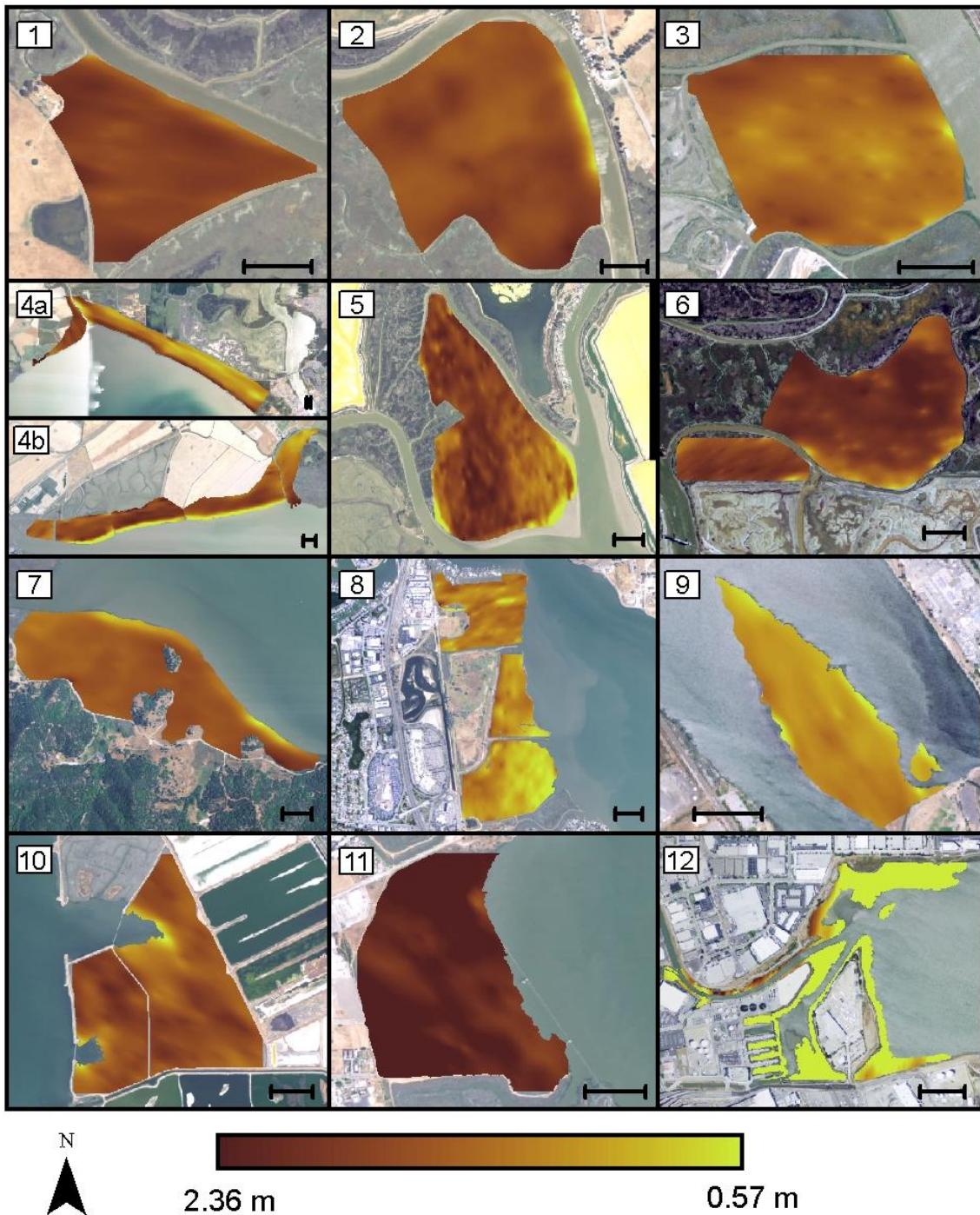
**Figure 6.** Elevation models for all marsh sites (NAVD88). Model parameters were optimized to reduce RMS. Scale bar = 200 m. 1 = Gambini, 2 = Petaluma, 3 = Black John, 4a = east San Pablo Bay NWR, 4b = west San Pablo Bay NWR, 5 = Coon Island, 6 = Fagan, 7 = China Camp State Park, 8 = Corte Madera, 9 = Arrowhead, 10 = Cogswell, 11 = Laumeister, 12 = Colma.
