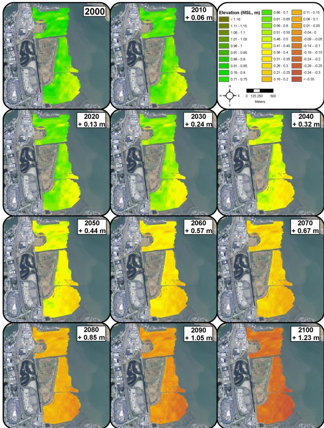
**Figure G-6.** WARMER results for Corte Madera. WARMER accounts for changes in relative sea-level, subsidence, inorganic sediment accumulation, above/below ground organic matter productivity , compaction, and decay. Non-linear sea-level rise projections for California were used (Cayan *et al.* 2009).
