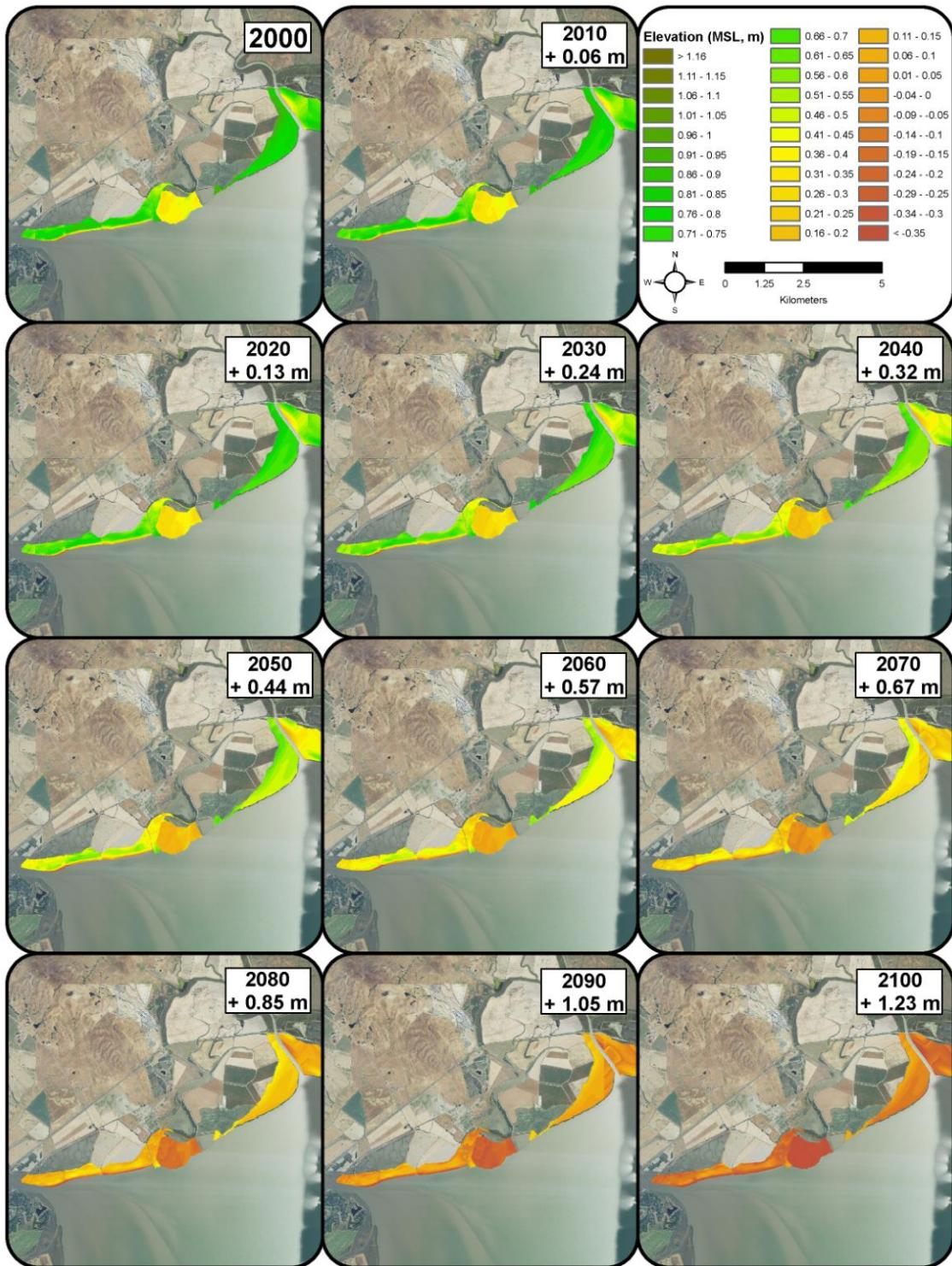
**Figure L-9.** WARMER results for west San Pablo. WARMER accounts for changes in relative sea-level, subsidence, inorganic sediment accumulation, above/below ground organic matter productivity, compaction, and decay. Non-linear sea-level rise projections for California were used (Cayan *et al.* 2009).
