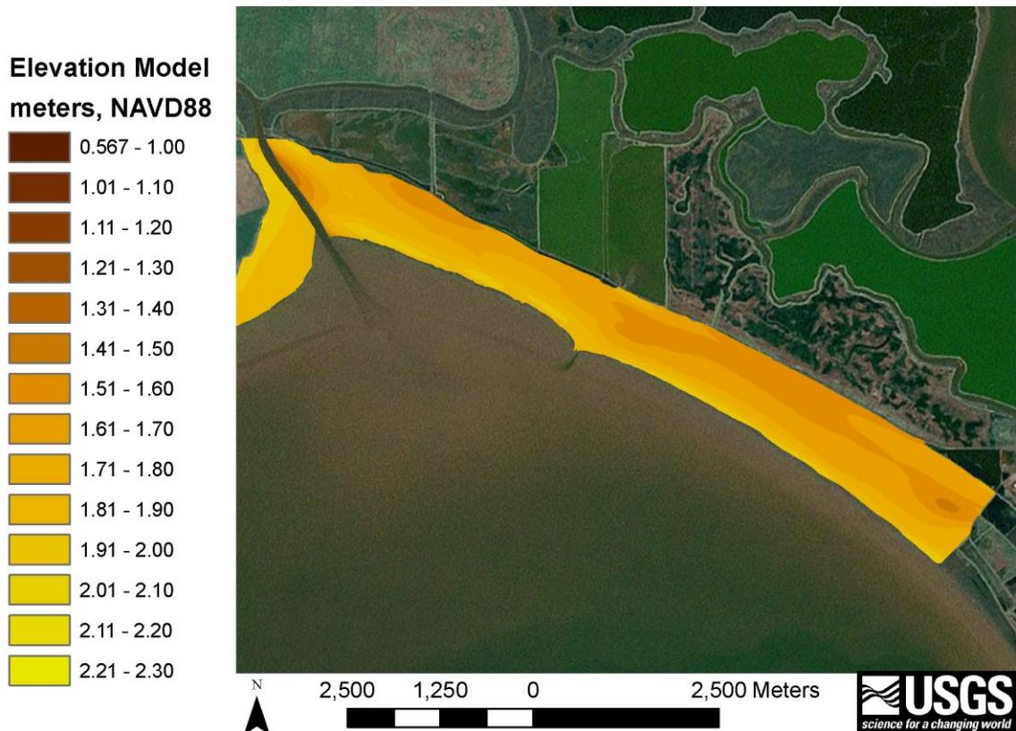
**Figure L-5.** Elevation model (3-m resolution) developed from ground RTK GPS elevation data for east San Pablo.
