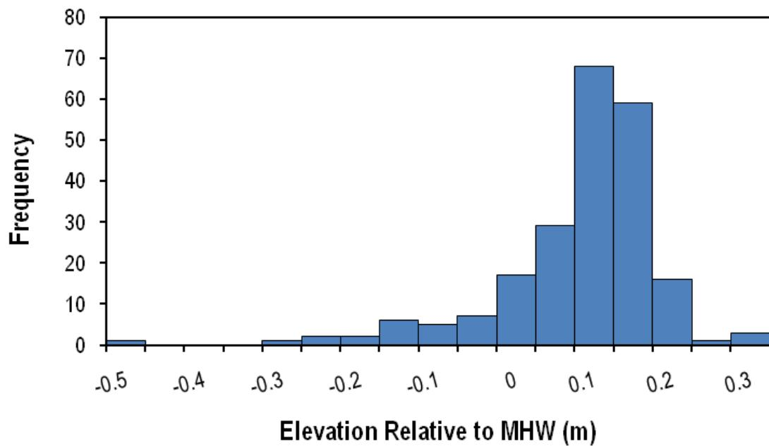
**Figure I-2.** Distribution of elevation samples relative to local mean high water (MHW) at Gambini marsh.
