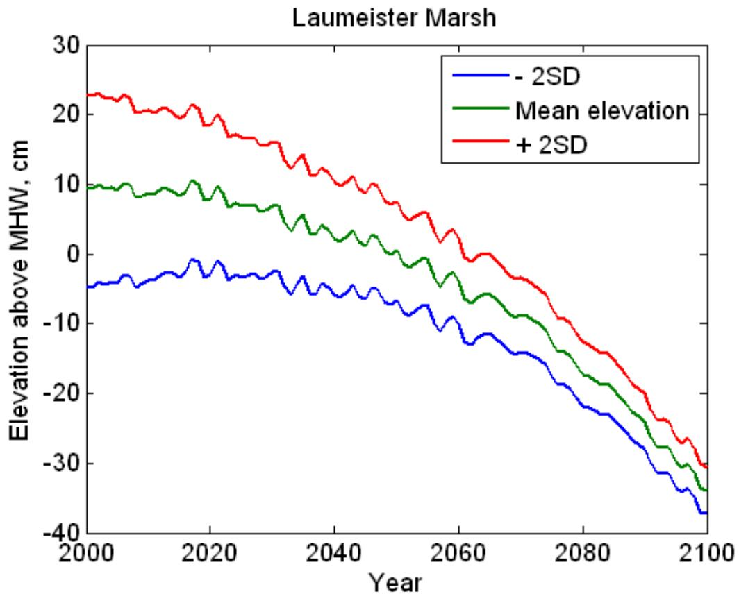
**Figure J-6.** WARMER scenarios of marsh elevation change for Laumeister. Elevation above MHW is plotted versus model year with two standard deviations (SD).
