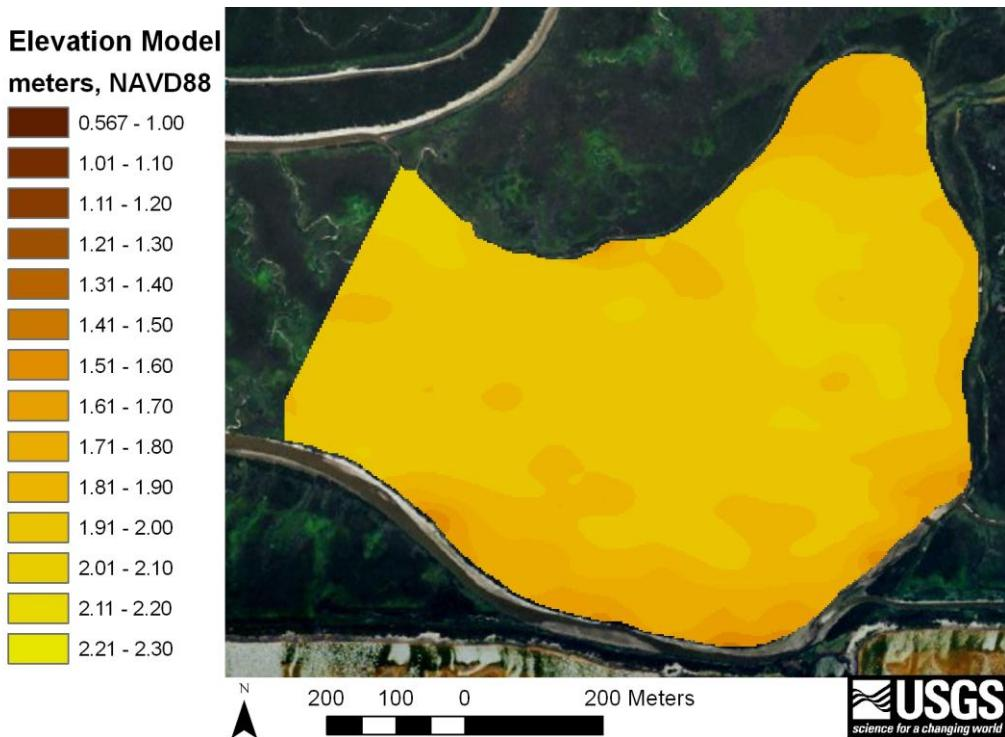
**Figure H-3.** Elevation model (3-m resolution) developed from ground RTK GPS elevation data.
