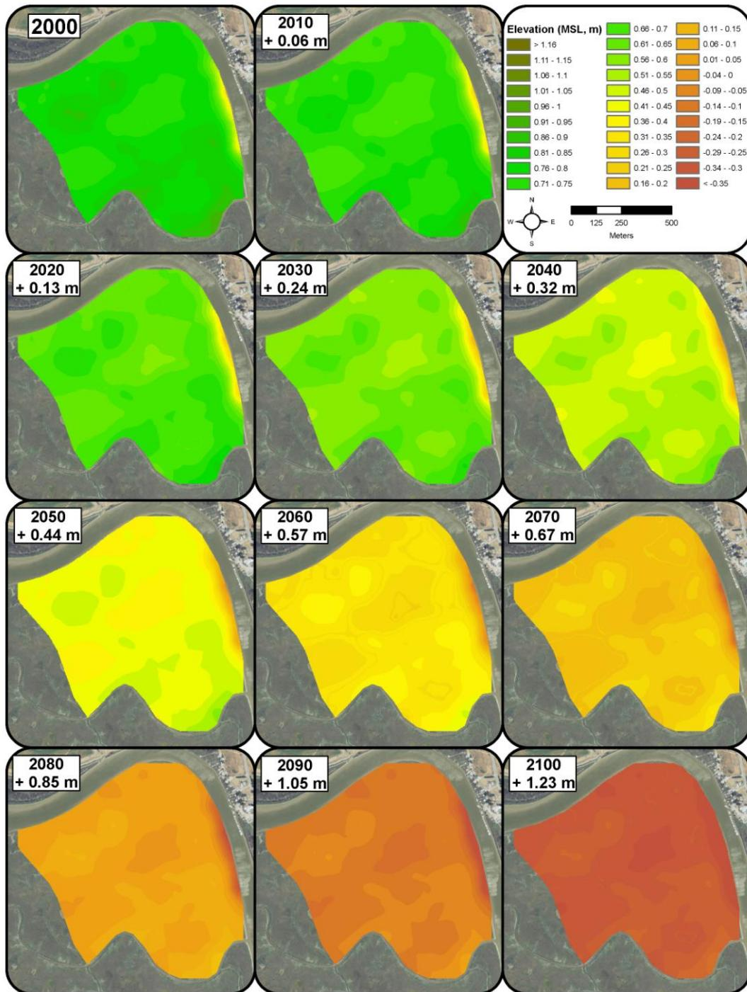
**Figure K-6.** WARMER results for Petaluma marsh. WARMER accounts for changes in relative sea-level, subsidence, inorganic sediment accumulation, above/below ground organic matter productivity, compaction, and decay. Non-linear sea-level rise projections for California were used (Cayan *et al.* 2009).
